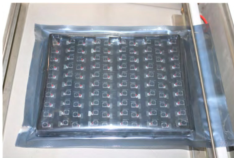
Vacuum the Anti-Static Bag
