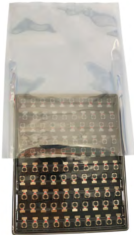
Place Tray into Anti-Static Bag
