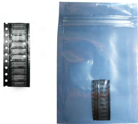
Place Connectors into Reel
